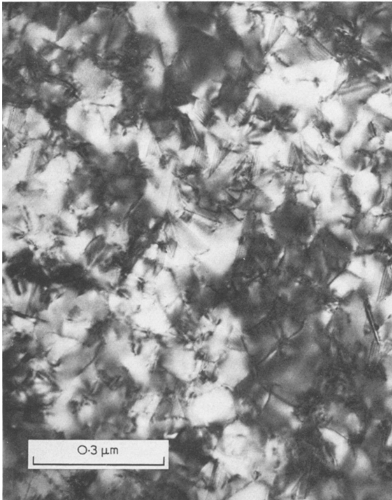
Figure 5 Transmission electron micrograph of a film of ZnTe grown on (111) Ge at 350°C.
